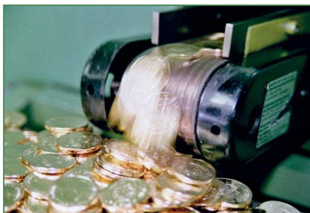
A minting machine at The Royal Mint can mint around 700 coins per minute. This machine and two others mint all the coins in circulation in Denmark. The coins are minted with a force of 35 to 90 tons, depending on size and thickness.
